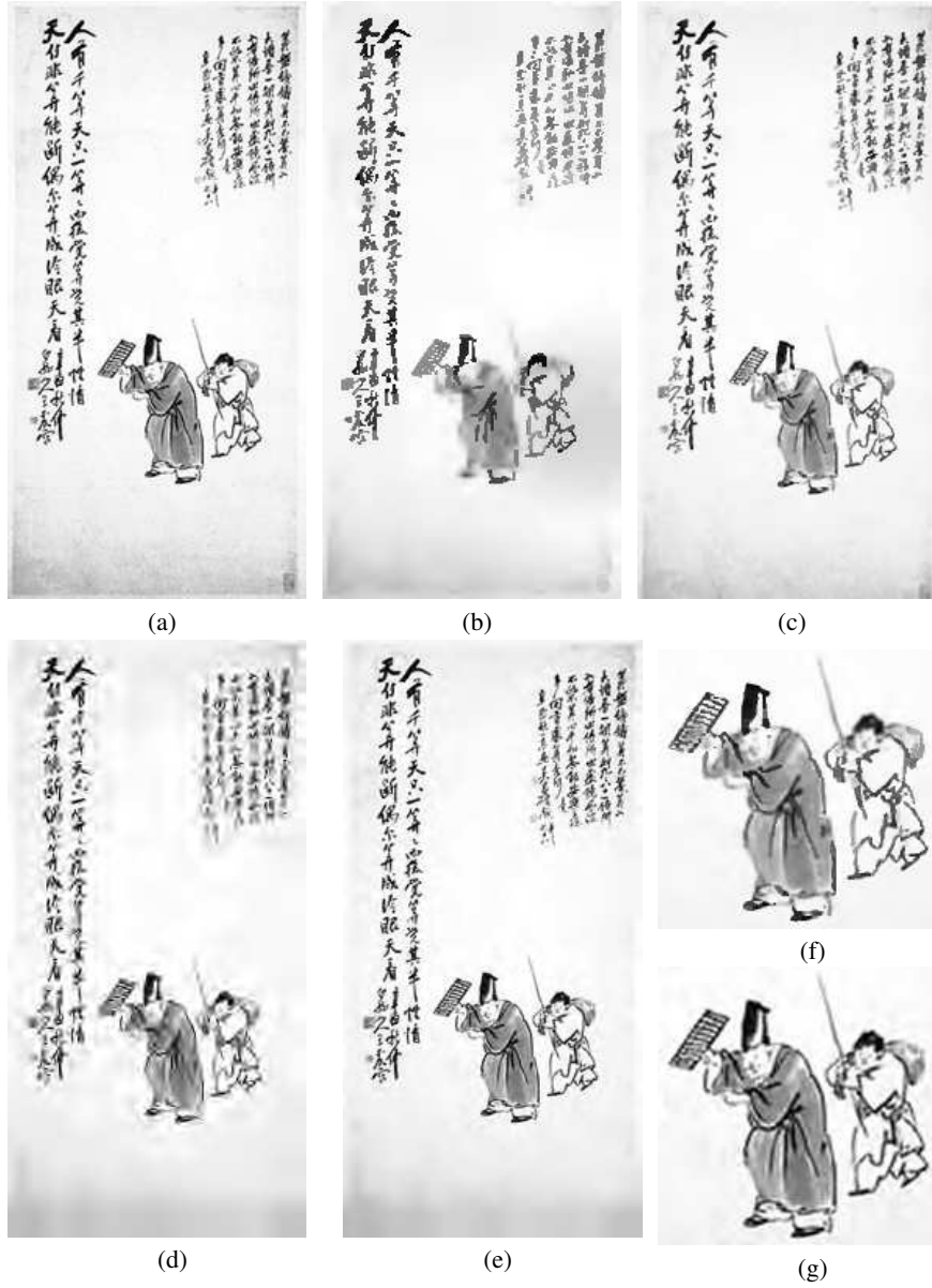
Fig. 6. Chinese ancient art: (a) original image (b) DjVu at 0.028 bpp (c) DjVu at 0.104 bpp (d) SPIHT_roi_max at 0.028 bpp (e) SPIHT_roi_max at 0.104 bpp (f) Zoomed in version of (c) (g) Zoomed in version of (e)
