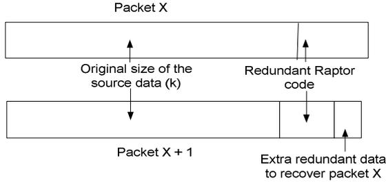
**Figure 3. Division of payload data in a packet (MPDU) between source data, original redundant data and piggybacked data for a previous errored packet.**
