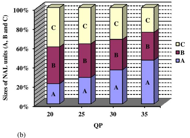
**Figure 1. Relative sizes of data partitions according to quantization parameter (QP) for the *Football* video sequence, with (a) 5% intra-coded refresh MBs, and (b) 25% intra-coded refresh MBs.**
