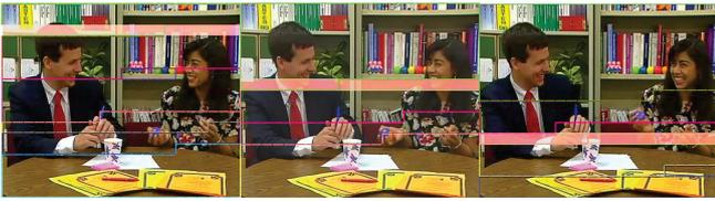
Fig. 1. Cyclic intra-refresh MB line technique for the *Paris* test sequence, showing successive MB lines in lighter shading, slice boundaries also shown.
