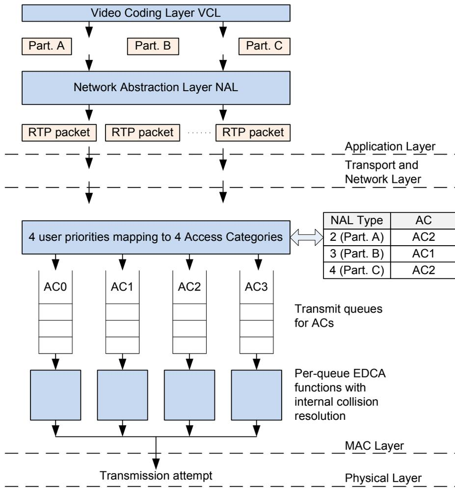
Fig. 7. IEEE 802.11e access category mapping for the data-partitioned packets.
