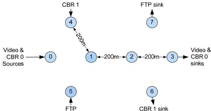
**Fig. 10.** Network topology used in our simulations.
