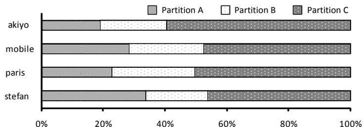
**Fig. 4.** Percentage of data for partitions A, B and C in a variety of sequences when an intra-refresh line is used.
