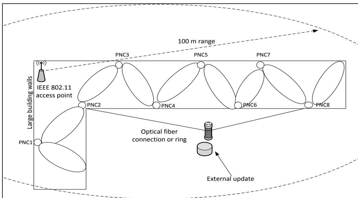
Figure 2 – Example large-building scenario for 60 GHz coverage
