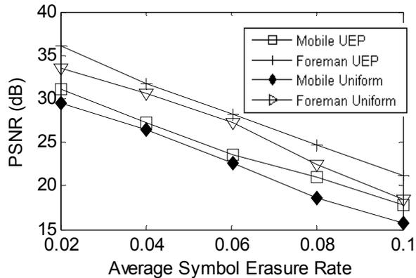
Fig. 3. Effect of UEP compared to uniform protection (EEP) for increasing symbol erasure lengths with an average error burst size of ten symbols for a G-E channel.
