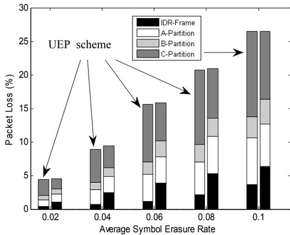
Fig. 5. Packet (NALU) loss distribution for the Mobile clip with average burst length of twenty symbols with UEP to the left and EEP to the right for a G-E channel.
