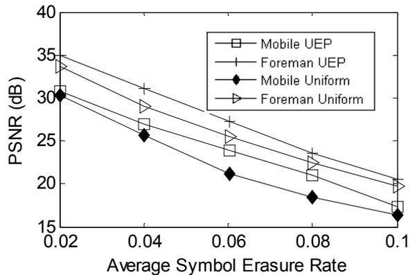
Fig. 4. Effect of UEP compared to uniform protection (EEP) for increasing symbol erasure rates with an average error burst size of twenty symbols in a G-E channel.
