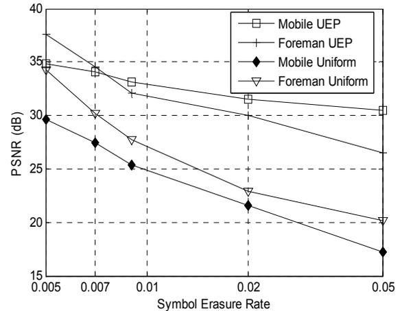
Fig. 6. Effect of UEP compared to uniform protection (EEP) for increasing symbol erasure rates with an average error burst size of twenty symbols in a REIN model channel.
