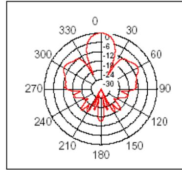
**Beam Angle:** Tested at 40.0Khz frequency
