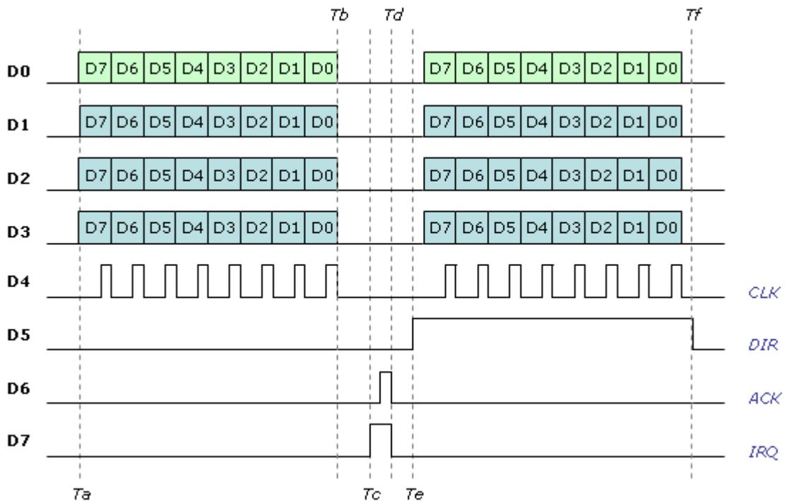
Figure 11: Timing diagram for the local bus.
