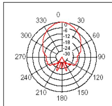
**Beam Angle:** Tested at 40.0KHz frequency
