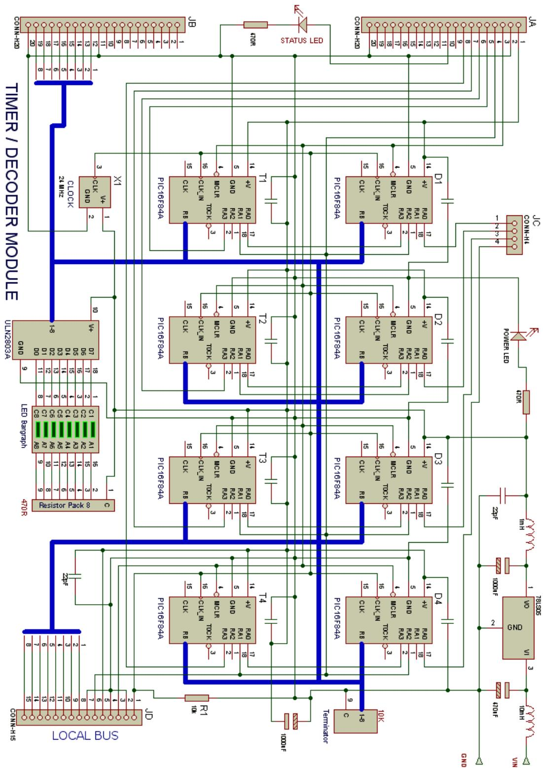
Figure 12: Circuit diagram for the decoder/timer board.
