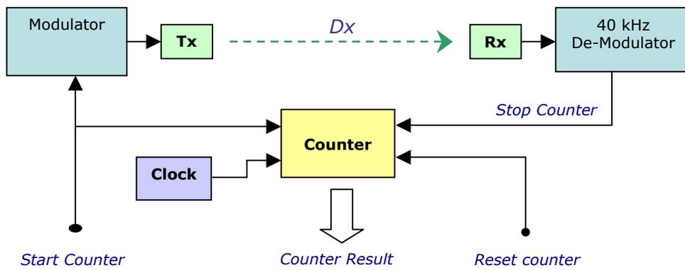
Figure 5: Measuring distance with ultrasound by means of a timer.
