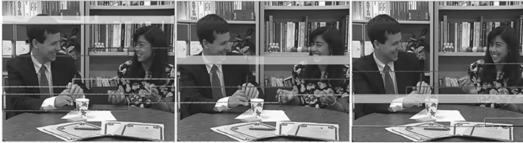
Figure 2. Cyclic intra-refresh MB line technique for the Paris test sequence, showing successive lines in lighter shading, with slice boundaries also shown.
