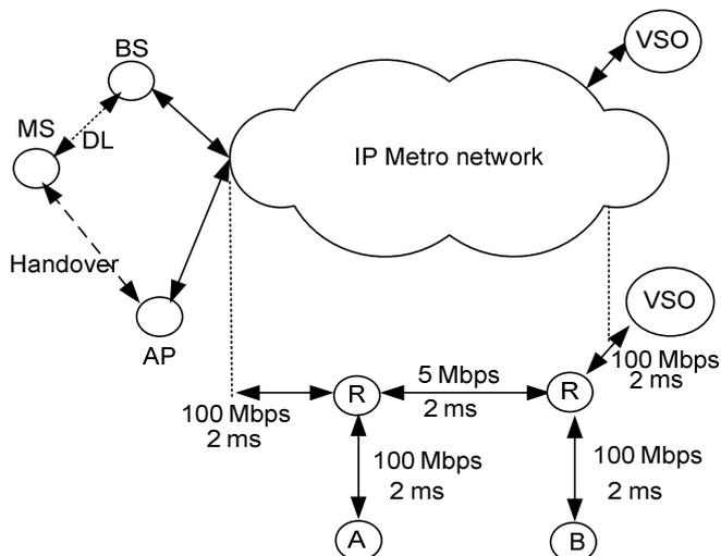
**Fig. 3.** Video streaming during the vertical handover scenario, MS = mobile subscriber station
