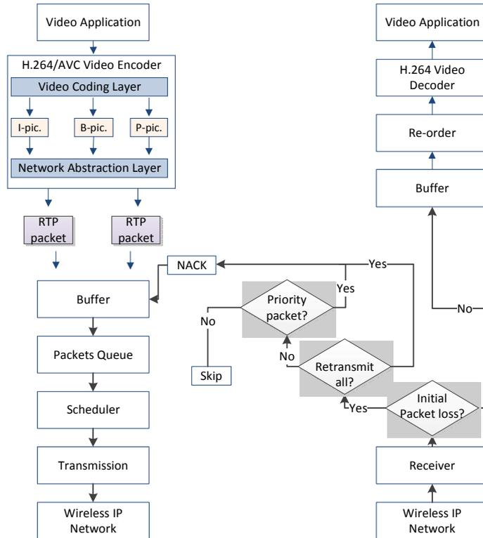
Fig. 2. Operation of BVS NACK enhancement to UDP
