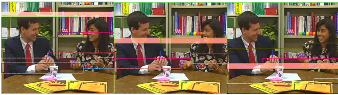
Fig. 1. Cyclic intra-refresh MB line technique for the Paris test sequence, showing successive MB lines in lighter shading, with some slice boundaries also shown.
