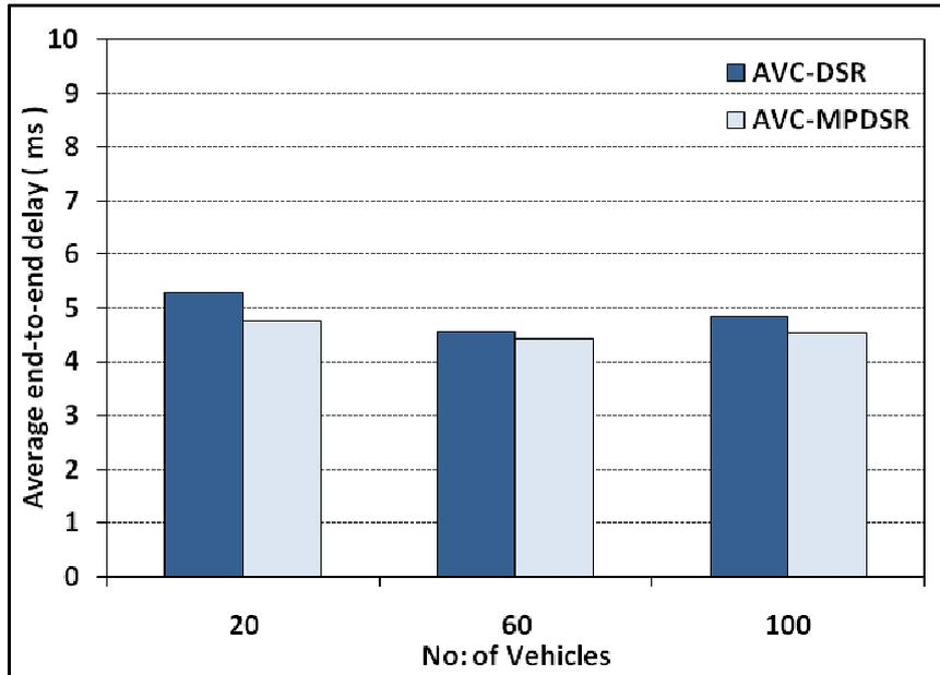
Figure 6. Comparison of the end-to-end delay between H.264/AVC unicast streaming (AVC) with single path routing using DSR and multi-path routing using MP-DSR
