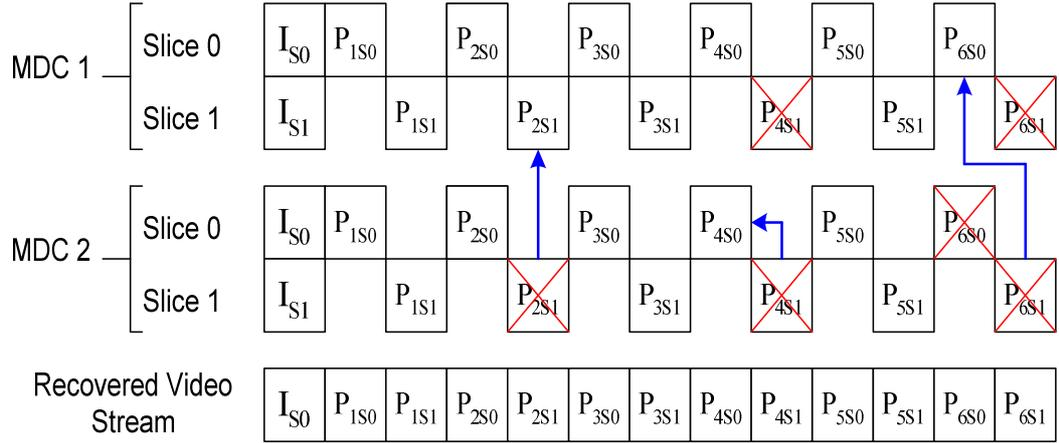
Figure 1. An example of the proposed slice compensation scheme with MDC and FMO, with arrows indicating the relationship “can be reconstructed from”
