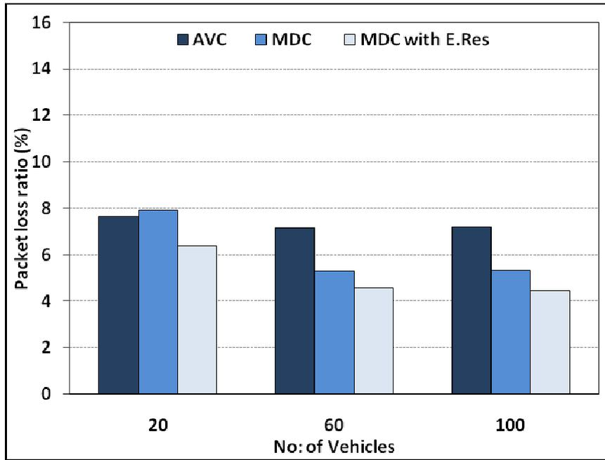
Figure 7. Comparison of the packet loss ratio between H.264/AVC unicast streaming (AVC), MDC and MDC with error resilience (MDC with. E. Res) with MDC schemes using MP-DSR
