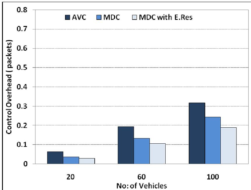
Figure 8. Comparison of the control packet overhead between H.264/AVC unicast streaming (AVC), MDC and MDC with error resilience (MDC with. E. Res) with MDC schemes using MP-DSR
