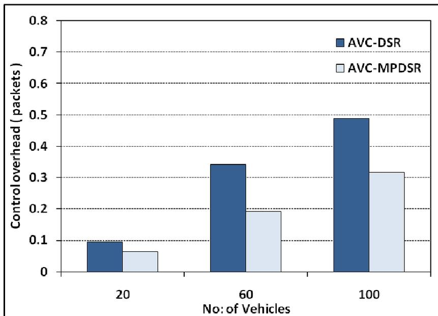
Figure 5. Comparison of the control packet overhead between H.264/AVC unicast streaming (AVC) with single path routing using DSR and multi-path routing using MP-DSR
