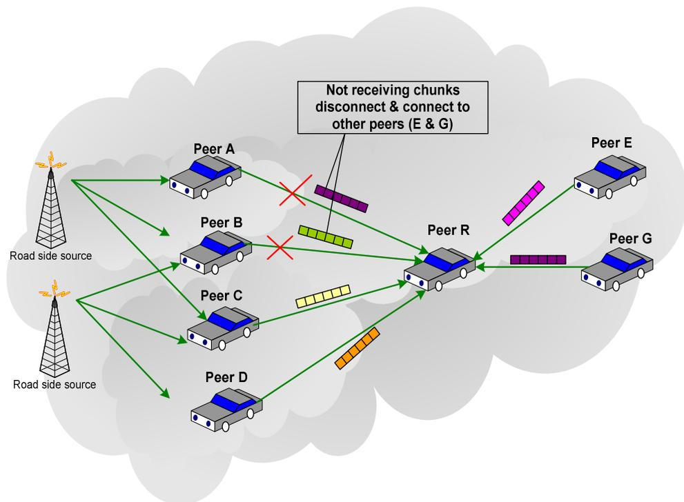
Figure 3. Mesh-based P2P topology sending video chunks from roadside sources to peers within the VANET, from which the chunks are distributed over multiple paths
