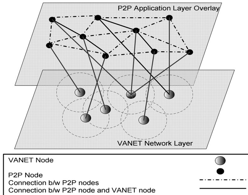
Figure 2. An example of a P2P application overlay over an ad hoc network, after [15]
