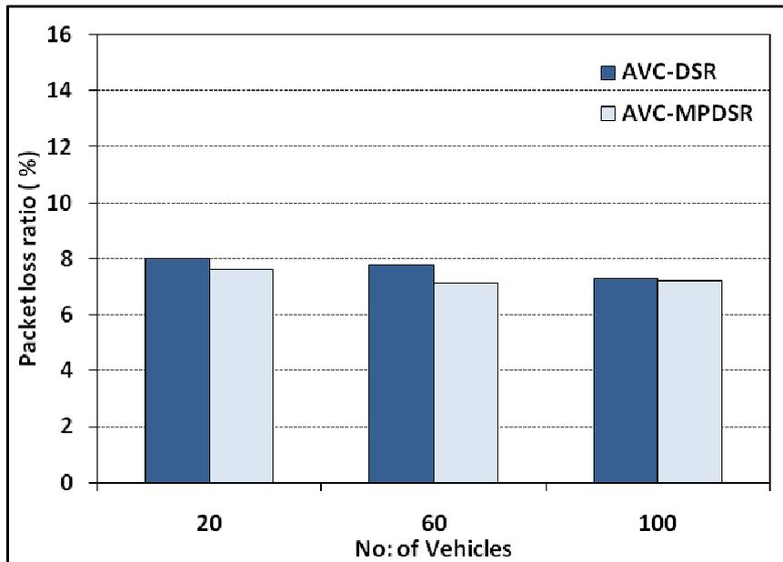
Figure 4. Comparison of the packet loss ratio between H.264/AVC unicast streaming (AVC) with single path routing using DSR and multi-path routing using MP-DSR
