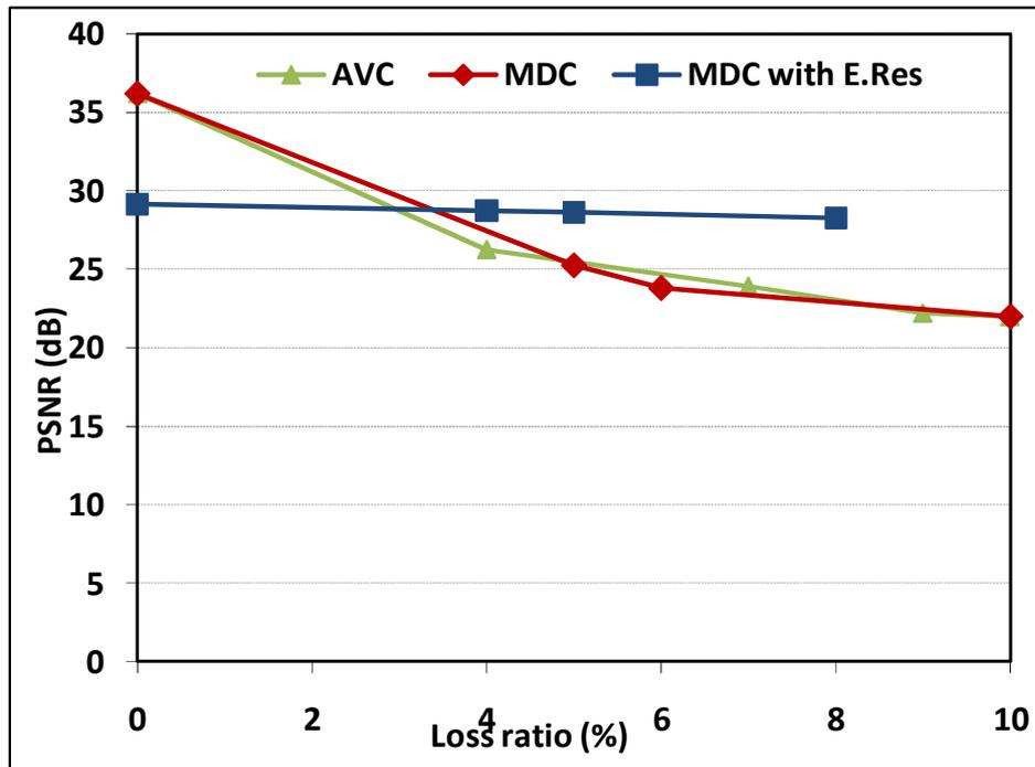
Figure 10. Comparison of the video quality between H.264/AVC unicast streaming (AVC), MDC and MDC with error resilience (MDC with. E. Res) with MDC schemes using MP-DSR
