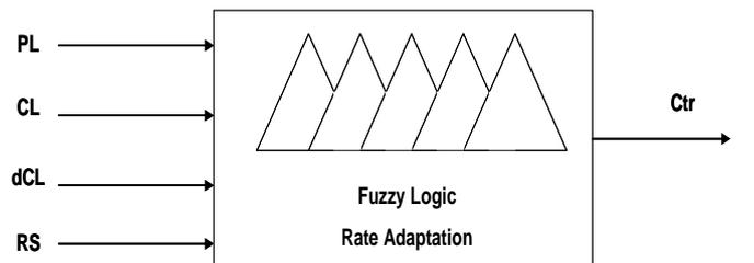
Figure 2: Block diagram depicting the inputs and outputs to a fuzzy congestion controller.
