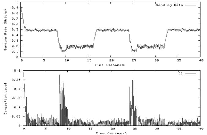
Figure 7: Graph showing the congestion level and sending rate of a 1Mbit/s CBR source adapting to a varying available bandwidth.
