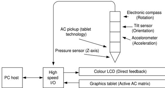
Figure 5: Block diagram of a direct-feedback interface
