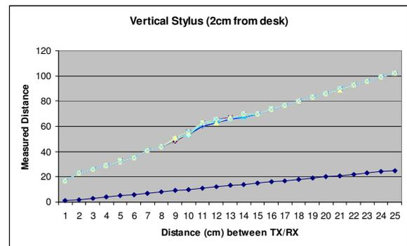
Figure 12: Wide-beam transmitter vertical response
