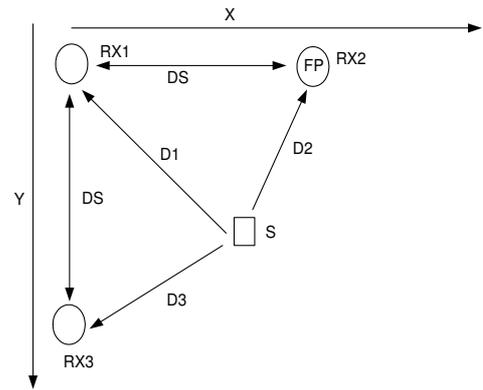
Figure 6: Triangulating the position of the stylus
