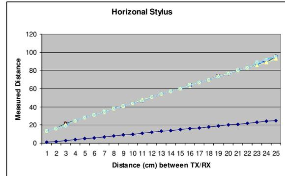
Figure 11: Wide-beam transmitter horizontal response
