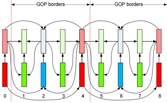
Fig. 2. Illustrative coding structure for GOP size of four with base and single enhancement layer, showing the prediction structure. Pictures appearing at 0, 4, and 8 are coded as key pictures
