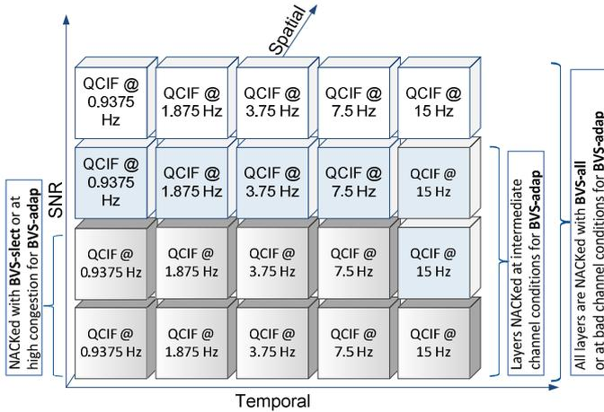
Fig. 3. H.264 SVC mapping to BVS-S. Packets belonging to darkly shaded layers are those that are negatively acknowledged
