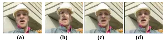
Figure 5. Frame with AODV routing and 15% error for (a) no error (b) single stream (c) VRC, and (d) redundant frames.
