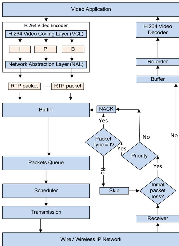
Fig. 3. Operation of selective NACK scheme
