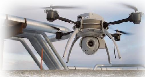
Fig. 1. Quadcopter showing camera and adjacent oil pipeline
