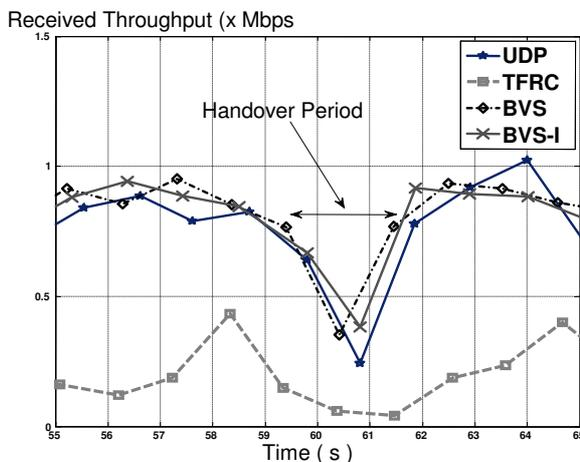
Fig. 4. Received data throughput during a handover
