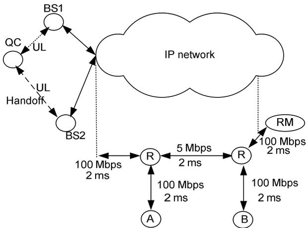
Fig. 2. Video streaming during handover scenario
