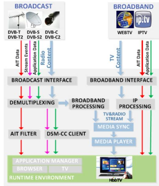
Fig. 2. Framework hybrid broadcast (audio Radio channel) and broadband (video IPTV channel) with Media Sync Module included
