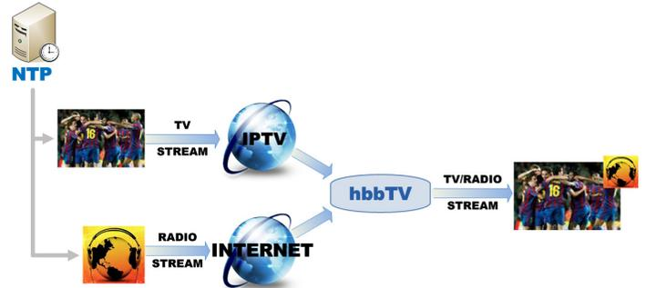
Fig. 1. Framework prototype to synchronise IPTV channel with Internet Radio via NTP synchronised sources to perform audio substitution at client-side
