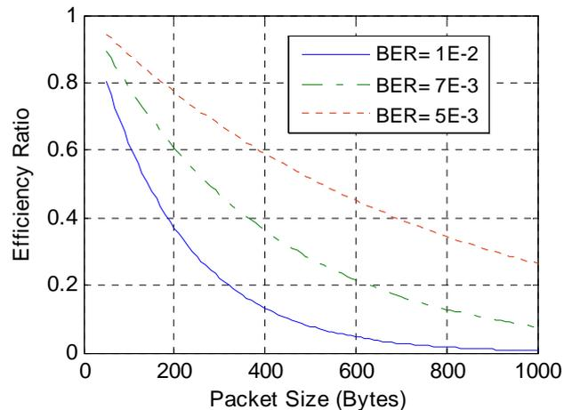
Figure 3: BER versus packet size for the transmission power efficiency of block based over packet-based single retransmission, both with FEC.
