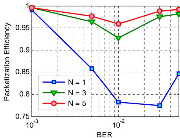
Figure 4: BER versus Bluetooth packet efficiency
