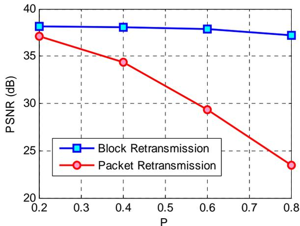
Figure 6: Video quality under packet and block retransmission, with varying ratio of bad state channel
