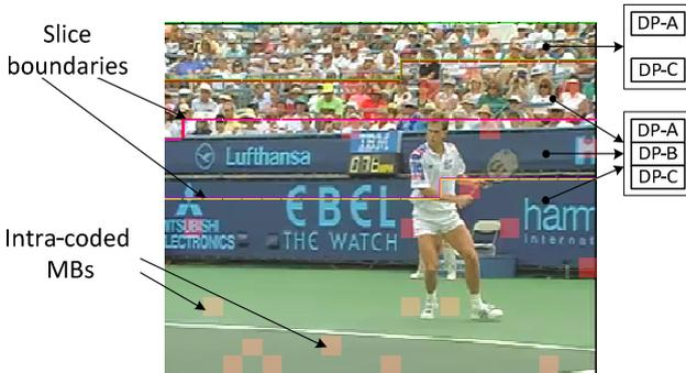
Figure 3. Example video frame from *Stefan* split into equal bit length slices, showing each slice partitioned into three partitions (A, B, C). Notice that it is possible in some circumstances for partitions B (or C) to be missing.
