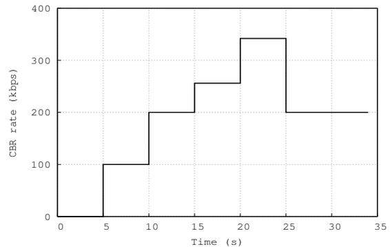
Fig. 2. Stepped CBR source acting as cross-traffic
