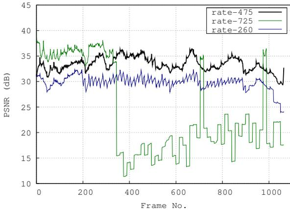
**Fig. 5.** CBR-encoded objective video quality (Y-PSNR) for HN video streaming at rates of 260, 475, and 725 kbps with UDP congestion
