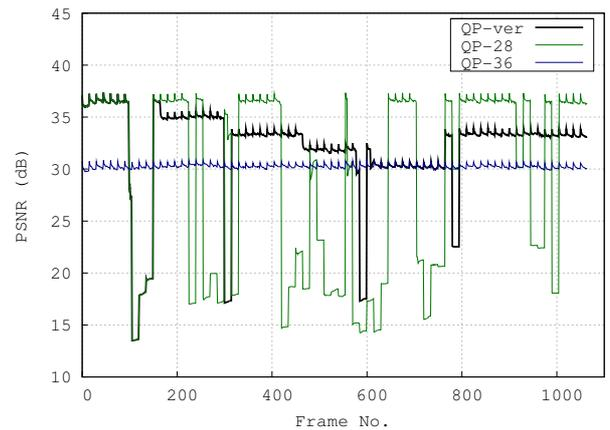
**Fig. 6.** VBR-encoded objective video quality (Y-PSNR) for HN video streaming at QP 28 and 36, and variable QP (QPver) with TCP congestion
