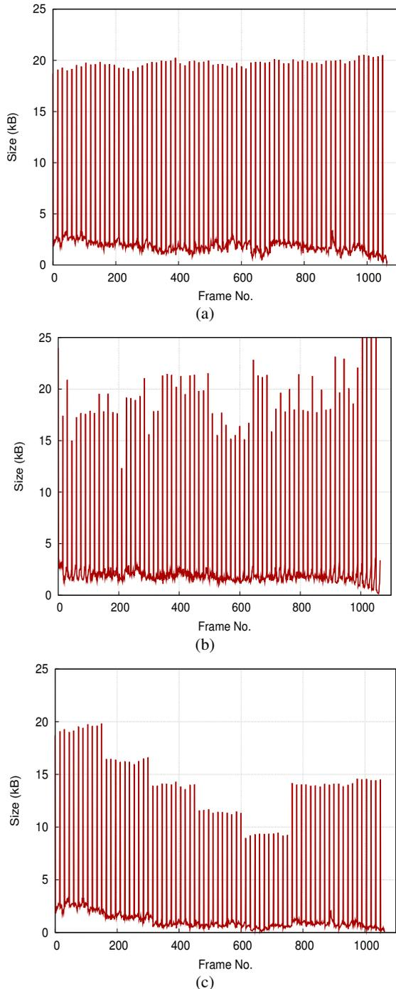
**Fig. 3.** Frame-by-frame compressed size for *Paris* in kbps for (a) higher-quality constrained VBR (QP=28), (b) CBR-encoded stream at 725 kbps, and (c) proposed variable quality VBR
