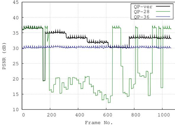
**Fig. 4.** VBR-encoded objective video quality (Y-PSNR) for HN video streaming at QP 28 and 36, and variable QP (QPver) with UDP congestion
