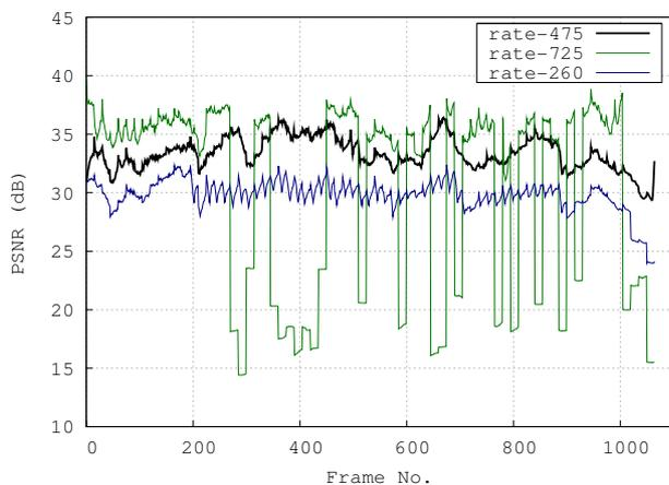
**Fig. 7.** CBR-encoded objective video quality (Y-PSNR) for HN video streaming at rates of 260, 475, and 725 kbps with TCP congestion
