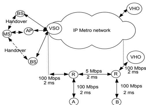
Figure 3. Video streaming scenario with dual handovers as video is streamed from the VHO
