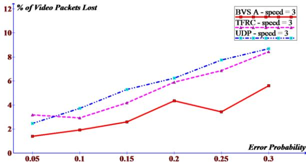
Figure 5 Packet Loss for Different Channel Conditions
