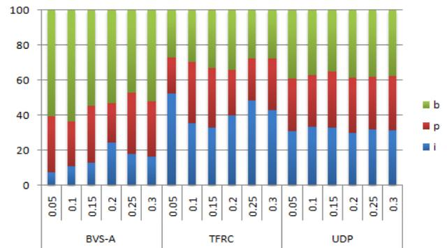
Figure 8 Frame type packet loss percentage for different channel conditions (PB = 0.05 ... 0.3) with a mobile speed of 3 mps.
