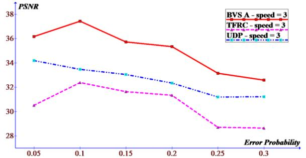
Figure 7 Video quality (Y-PSNR) of BVS-A for different channel conditions.
