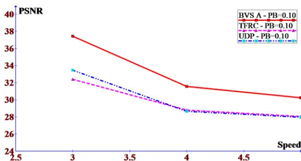
Figure 6. Video quality (Y-PSNR) of BVS-A for varying mobile device speeds.
