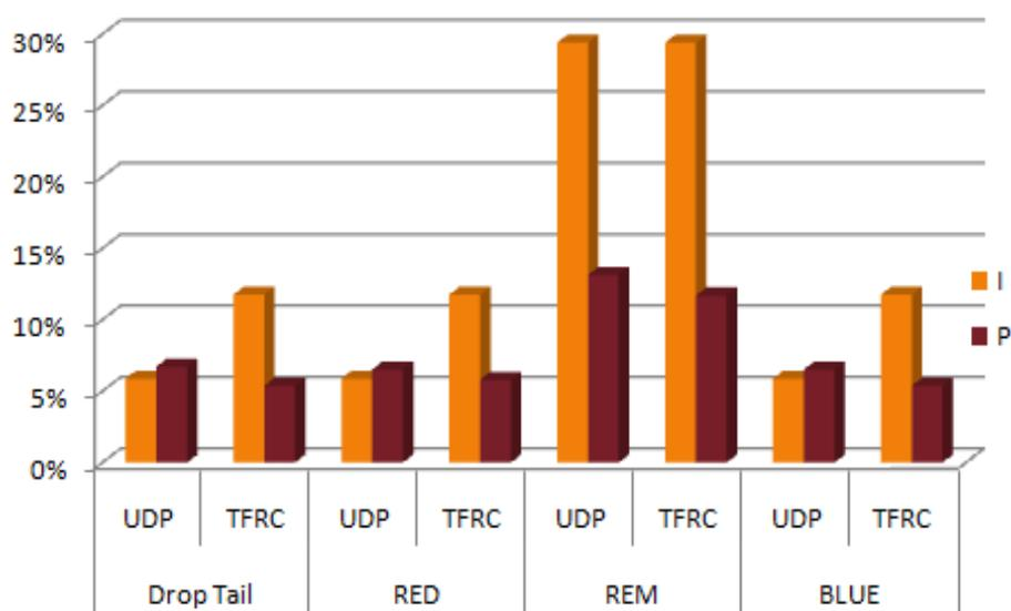
Figure 13. Percentage of I- and P-frame packets dropped relative to numbers of I- and P-frame packets respectively.
