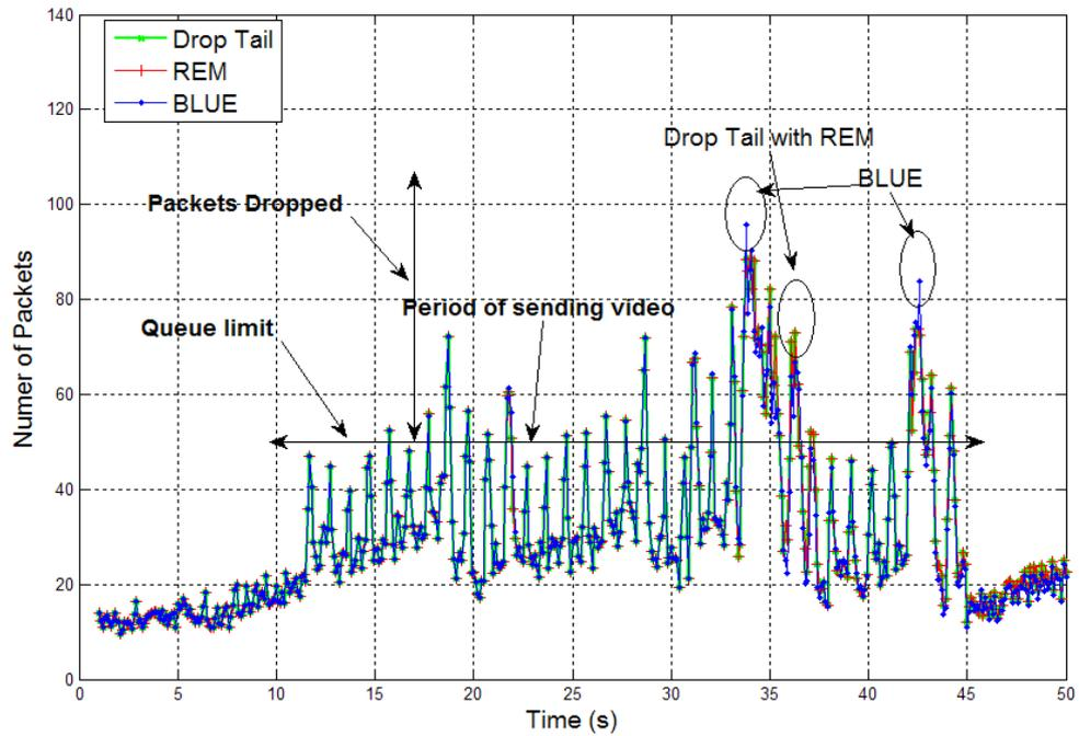
Figure 5. Buffer occupancy and packet drops for UDP transport, with drop-tail, REM and BLUE queuing disciplines.
