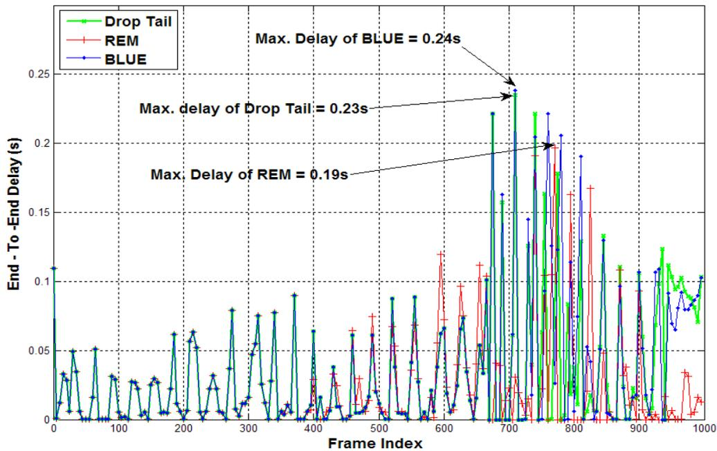
Figure 11. Delay over time (frames) for TFRC transport with drop-tail, REM and BLUE queuing disciplines.
