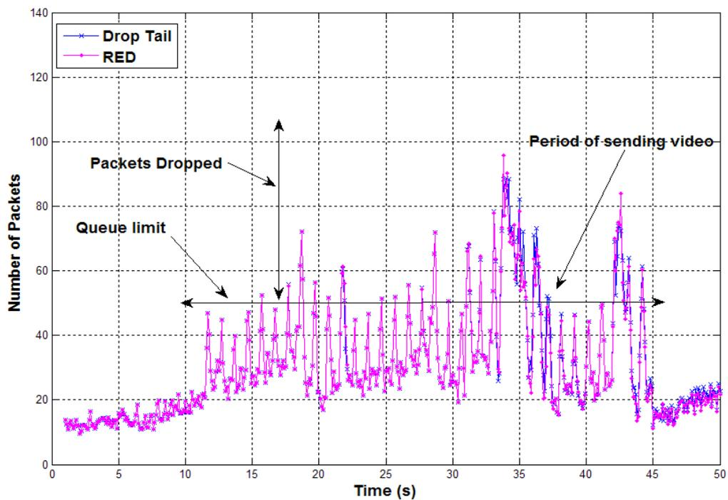
Figure 6. Buffer occupancy and packet drops for UDP transport, with drop-tail and RED queuing disciplines.
