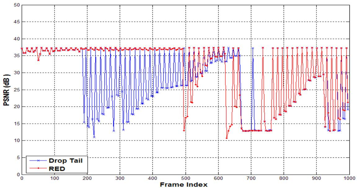
Figure 8. PSNR over time (frames) for UDP transport with drop-tail and RED queuing disciplines.
