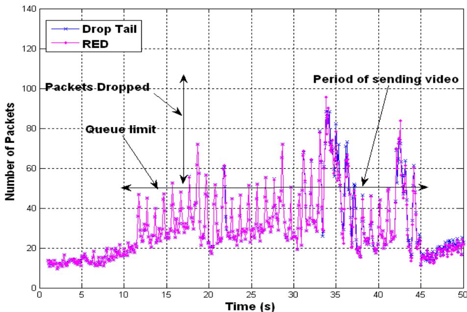
Figure 10. Buffer occupancy and packet drops for TFRC transport, with drop-tail and RED queuing disciplines.
