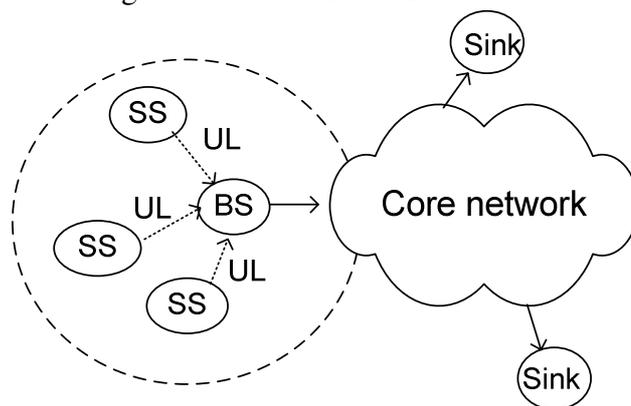
Figure 1. IEEE 802.16 uplink service architecture
