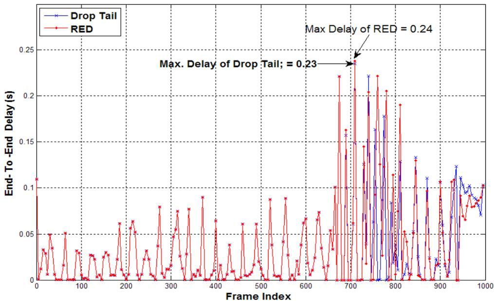
Figure 12. Delay over time (frames) for TFRC transport with drop-tail and RED queuing disciplines.
