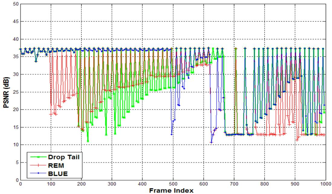
Figure 7. PSNR over time (frames) for UDP transport with drop-tail, REM and BLUE queuing disciplines.
