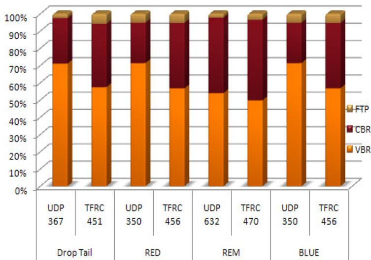
Figure 4. Percentage packet drops according to traffic type and transport for differing queuing disciplines.
