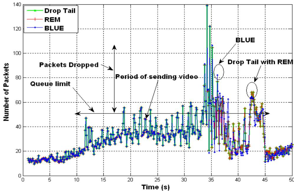
Figure 9. Buffer occupancy and packet drops for TFRC transport, with drop-tail, REM and BLUE queuing disciplines.
