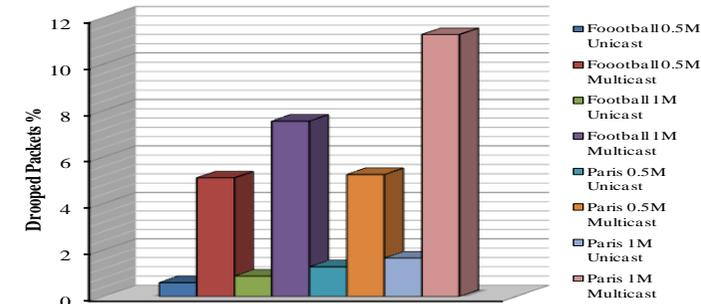
Fig.(3) Packet drop rates for unicast and multicast with adaptive Raptor coding. 0.5M= 0.5Mbps, 1M = 1 Mbps.
