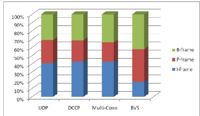
Figure 4. Breakdown by frame type of packet losses when downlink streaming
