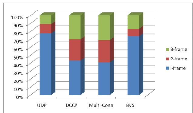
Figure 5. Breakdown by frame type of packet losses when uplink streaming
