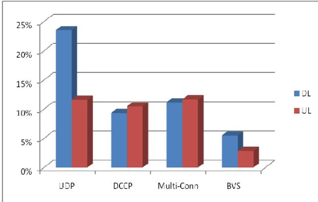
Figure 2. Percentage overall packet loss according to streaming direction.
