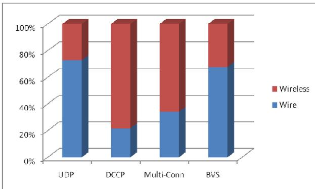
Figure 3. Proportion of wired/wireless network packet losses for downlink streaming.
