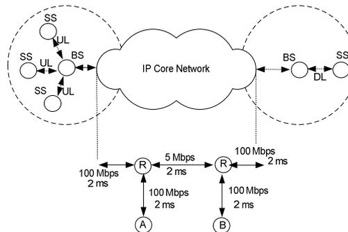
Figure 8. Network extension of Figure 1, with additional wireless downlink to mobile user.
