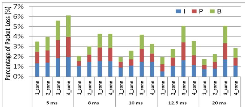
Figure 3. Mean percentage packet loss broken down according to frame type, by connection and TDD frame length, I = Intra-coded frame, P = Predictively-coded frame, B = Bi-predictively coded frame.
