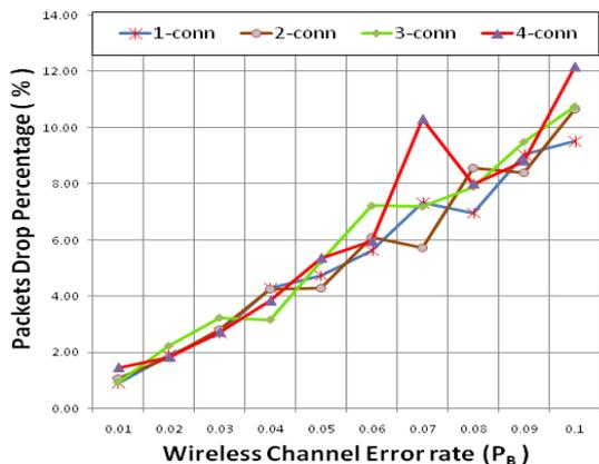
Figure 7. Packet drop rate with increasing probability of error in the Gilbert-Elliott bad state ( $P_B$ ).
