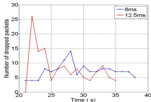
Figure 6. Packet drops over time for two selected frame sizes for four connections.
