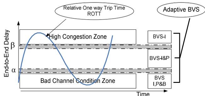
Fig. 1. The Spike scheme applied to BVS-A.
