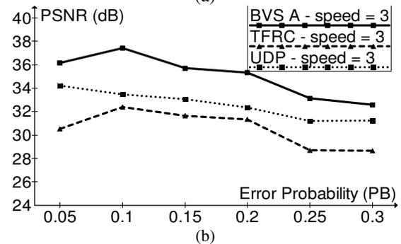
Fig. 3. Video quality (Y-PSNR) of BVS-A for (a) varying mobile device speeds (b) different channel conditions.
