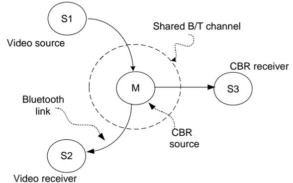
Figure 3. Scenario 2 with B/T piconet before dynamic reconfiguration.
