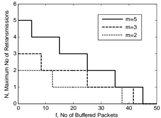
**Figure 2. Maximum number of retransmissions, RTO according to sender buffer fullness.**
