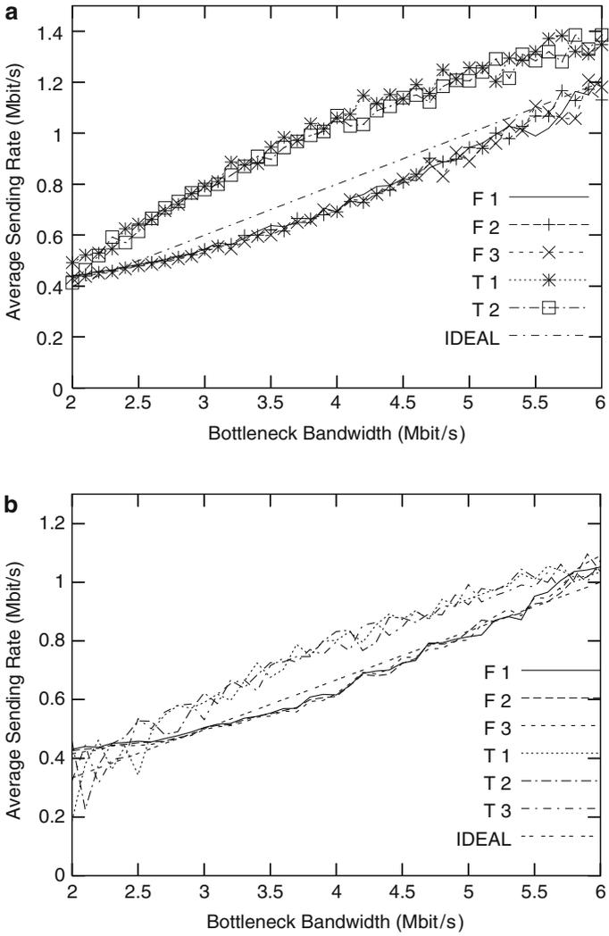
**Fig. 3.5** Multiple competing flows with different controllers across a range of bottlenecks, compared to an ideal per-flow allocation of bandwidth (a) 3 FLC and 2 TFRC flows (b) 3 FLC and 3 TFRC flows
