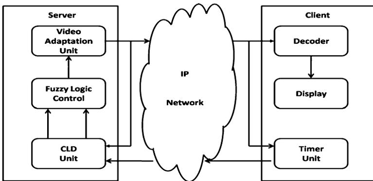
Fig. 3.1 Fuzzy logic control (FLC) video streaming architecture
