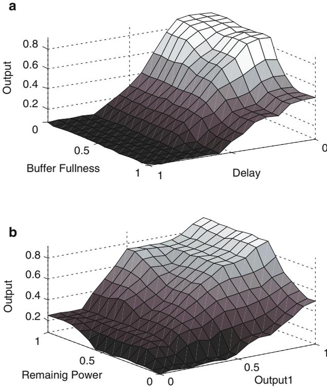
**Fig. 3.7** (a) Stage 1 FLC control surface resulting from FLC ARQ (b) Stage two control surface giving the transmission count output (before subsequent scaling)
