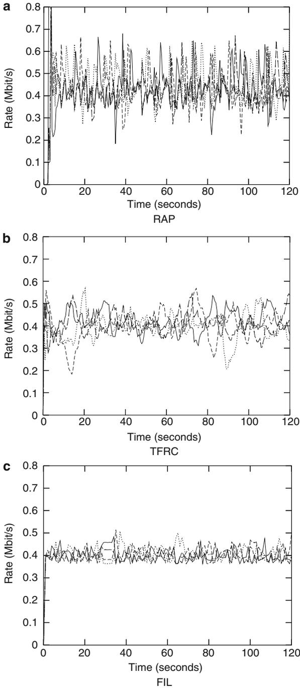
**Fig. 3.4** Five simultaneous flows each with identical congestion controllers for a 2 Mb/s bottleneck with (a) rate adaptation protocol controllers, (b) TCP-friendly rate control (TFRC) controllers, and (c) with FLC
