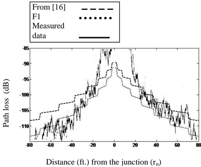
Fig. 5. Comparison of the equations for side-street path loss, from [16] and the revised equation (F1) including accurate calculation of propagation distance, ‘foliage’ effect, with measured data from [28], settings — frequency = 1.8 GHz,  $r_m = 110$  m,  $W_m = 20$  m,  $W_s = 26$  m,  $s = 0.002$
