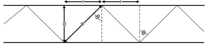
Fig. 2. Geometry for calculating reflection distance,  $R$
