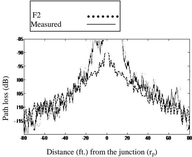
Fig. 6. Comparison of the equations for side-street path loss, the revised equation (F2) including accurate calculation of propagation distance, ‘foliage’ effect, and phase change, with measured data from [28], settings — frequency = 1.8 GHz,  $r_m = 110$  m,  $W_m = 20$  m,  $W_s = 26$  m,  $s = 0.002$
