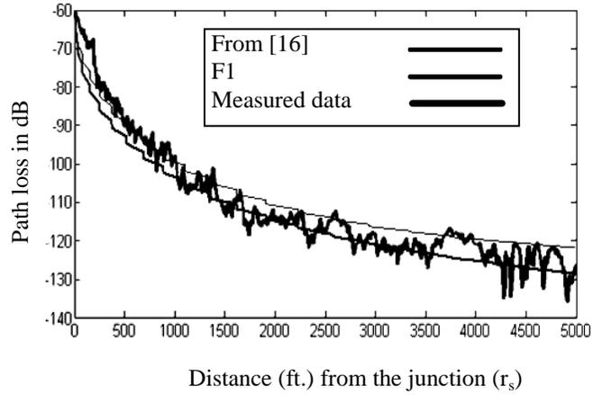
Fig. 3. Comparison of the equations for side-street path loss, from [16] and the revised equation (F1) including accurate calculation of propagation distance and ‘foliage’ effect, with measured data from [22], settings — frequency = 900 MHz,  $rm = 39.2$  m,  $Wm = 28.6$  m,  $Ws = 20.4$  m,  $s = 0.001$
