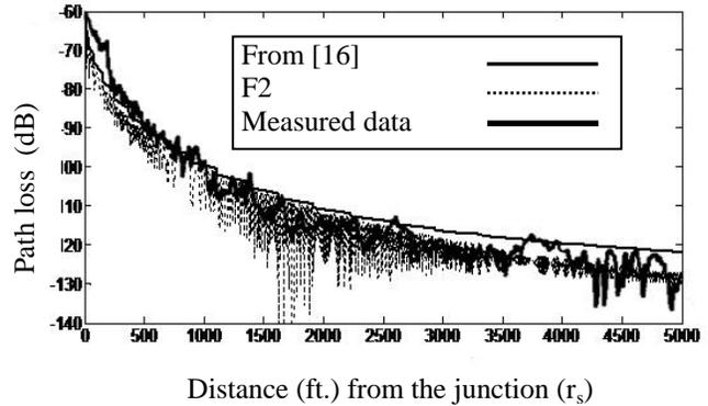
Fig. 4. Comparison of the equations for side-street path loss, from [16] and the revised equation (F2) including accurate calculation of propagation distance, ‘foliage’ effect, and phase change, with measured data from [22], settings — frequency = 900 MHz,  $rm = 39.2$  m,  $Wm = 28.6$  m,  $Ws = 20.4$  m,  $s = 0.001$
