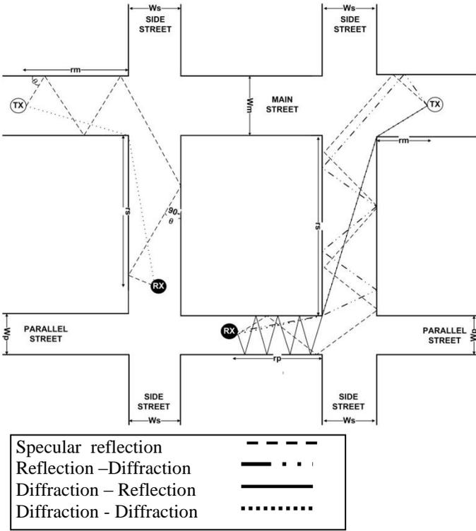
Fig. 1. Transmission paths from a transmitter (tx) to a receiver (rx) in a side street and from a transmitter and receiver in a parallel street.
