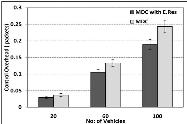
Fig. 5. MDC per packet overhead by VANET size with and without error resilience (E. Res) showing 95% confidence intervals
