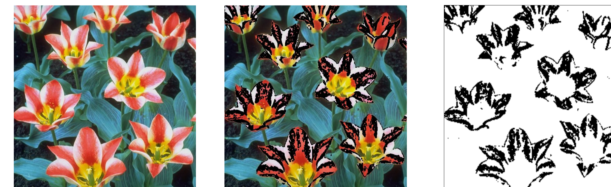
Left to right: original image; edge detected image; binary edge image.
